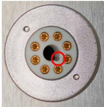
Tube socket guide pin indicator
