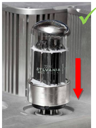
Insert a tube perpendicular to the socket.
