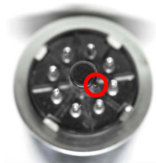
Guide pin shows on the bottom of a tube.
