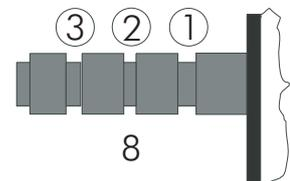
Hang the loop of the thread of the anti-skating weight (5) in the groove of the anti-skating stub (8) corresponding to the downforce applied to your cartridge and hang the thread in the groove of the wire support (6).
