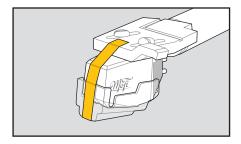
Install the cartridge stylus guard and use a small piece of tape to hold it in place.
