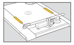
Attach two foam strips across the front and back of turntable.
