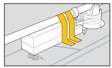
Secure tonearm with twist tie. Support tonearm base with foam blocks. Attach two strips of tape across top of tonearm over foam blocks and onto the top of turntable.
