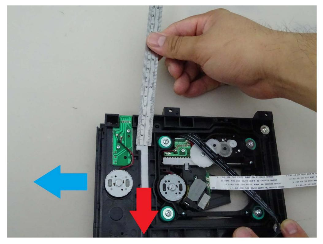
Step 4: Once the stuck CD is removed, push back the CD tray, reassemble the top cover.
