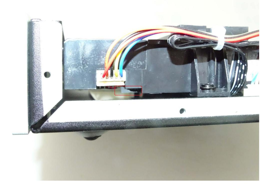
Step 3: Make sure the power is not connected, use a flat head screw driver or a flat ruler and push the white sliderdown. This will force the CD tray to eject.
