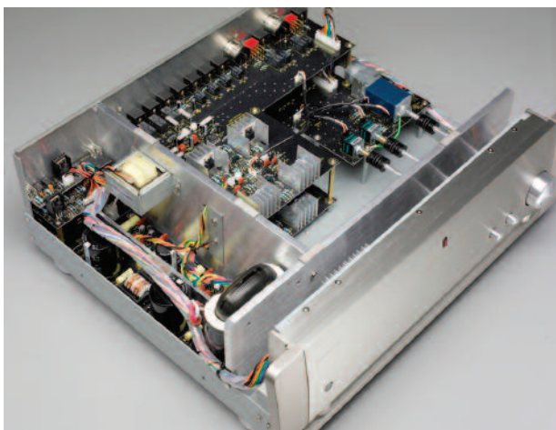
The JC 2's interior is divided into three by sheet aluminum partitions.
