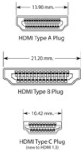
Fig.4 HDMI plug types
