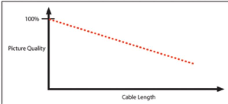
Fig.5 Picture quality of an analog single gradually declines over longer length of cable.
