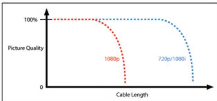
Fig.13 The edge of the "cliff" of a given cable varies by signal rate. The max distance of 1080p is only 1/2 of 1080i.
