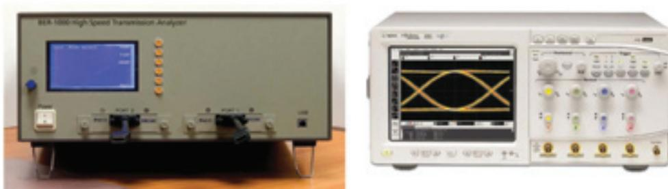
Fig.12 BER and Eye Pattern test equipment.
