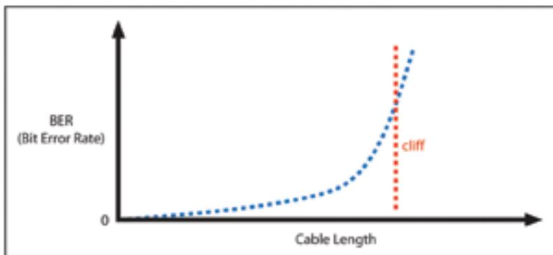
Fig. 8 BER (Bit Error Rate) test counts the number of error data at the far end of the cable. the "cliff" effect is visible.
