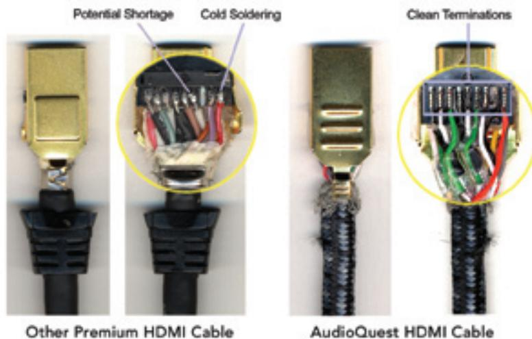
Fig.16 Soldering vs. crimped connection
