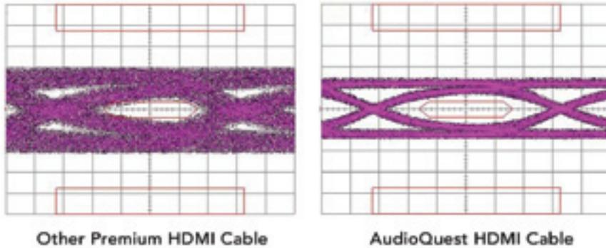
Fig.14 Eye pattern test results
