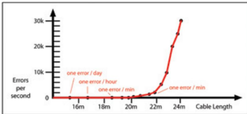
Fig.11 BER test also shows the “cliff” effects.
