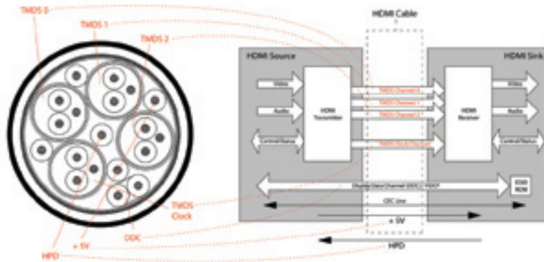
Fig.1 Inside an HDMI cable
