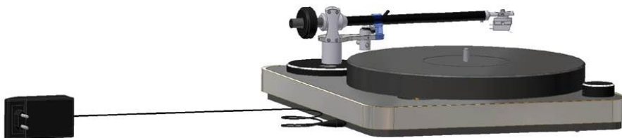
Pic. 7: Connecting the Power supply
